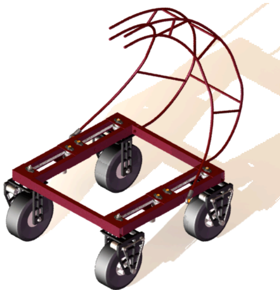
Figure 3 CAD rendering of Gladiator's chassis and tail
